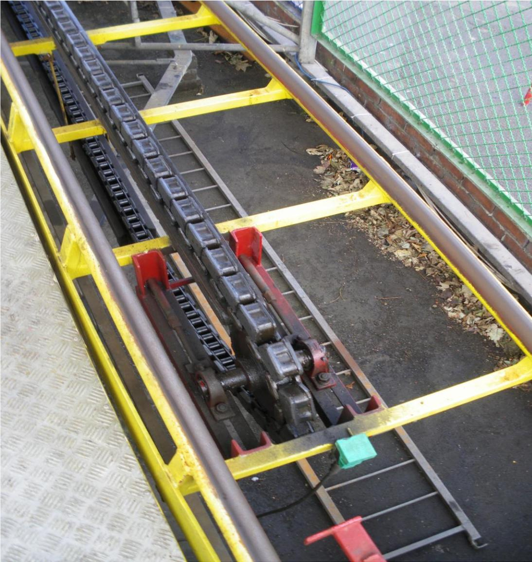
The sensor was set to operate the secondary air brake when the car passed it and functioned when a piece of metal plate attached to the car passed within 40mm of it.
