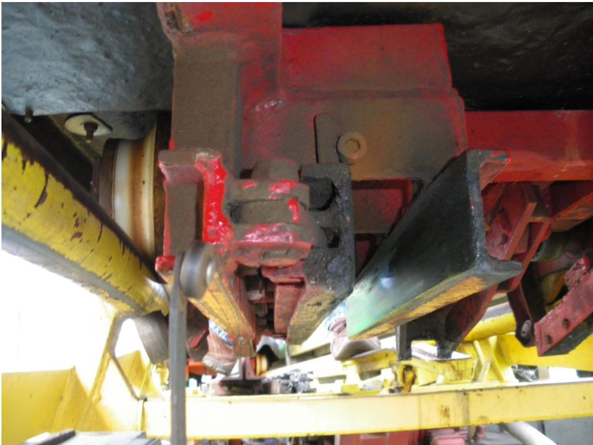
Early indications from the investigation suggest that the secondary air brake did not come on because the sensors were not functioning correctly and did not recognise the car passing them. The sensor was fixed at a suitable distance from the plate on the passing car.
