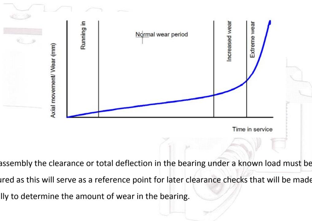
After assembly the clearance or total deflection in the bearing under a known load must be measured as this will serve as a reference point for later clearance checks that will be made at least annually to determine the amount of wear in the bearing.
