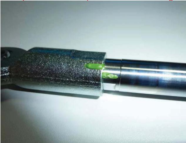
All units should be inspected daily during use. If the paint marking is discovered broken or if the joint head is not completely screwed in, the unit should not be used because the Personal Restraint System may fail possibly leading to personal injury or death of a rider.
