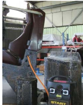
Test Box Connection on Coaster Vehicle
