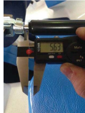
Lap bar closed position – creep measurement
