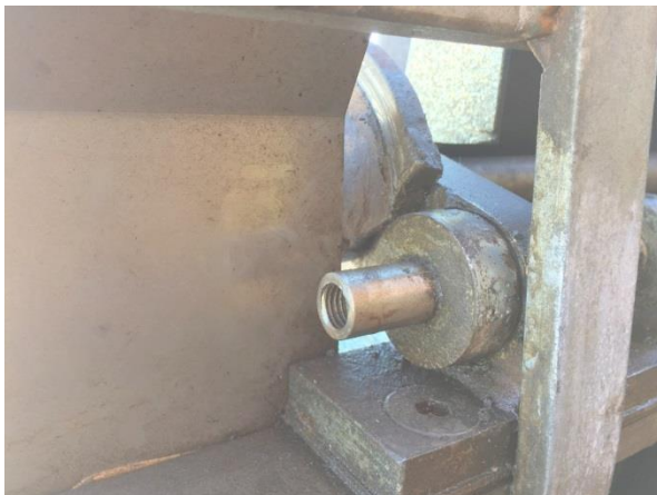
Note wear to cam plate due to harness being able to be raised before lateral movement has completed
